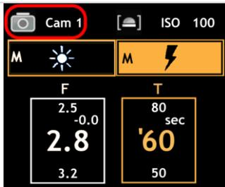
The selected user pre-set appears on the display. One of the following users can be selected: **Cam 1**, **Cam 2**, **Cam 3** or **Movie**.
