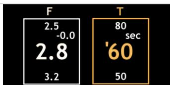
F-stop and time series can be gradated in accordance with your camera in steps of **1 EV**, **1/2 EV** and **1/3 EV**. This setting influences the f-stop and time series on the display.
