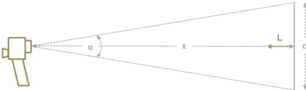
Diameter  $d$  of the measuring circle can be calculated from measuring angle  $\alpha$  and distance  $x$  with the help of the following trigonometric function:
