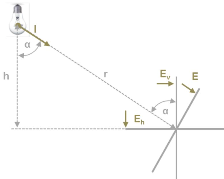
If the illuminated surface is laterally offset relative to the source of light, i.e. if the light does not strike the surface at a right angle, illuminance is reduced. If the light source is located at height  $h$  above the horizontal plane and angle of radiation  $\alpha$  makes reference to the vertical, horizontal illuminance  $E_h$  and vertical illuminance  $E_v$  are calculated as follows:
