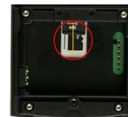
Insert micro SDHC card and push into the slot.
